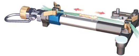
Graft is pretensioned at 300 - 500 Newtons for 30 - 60 seconds using the CoLS Tensor
